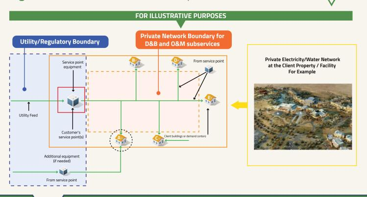
**Figure 1** shows an illustrative diagram depicting the private network of the client with the proposed boundaries for the Design, Build, Operations, Maintenance, and network CRM subservices scope.
